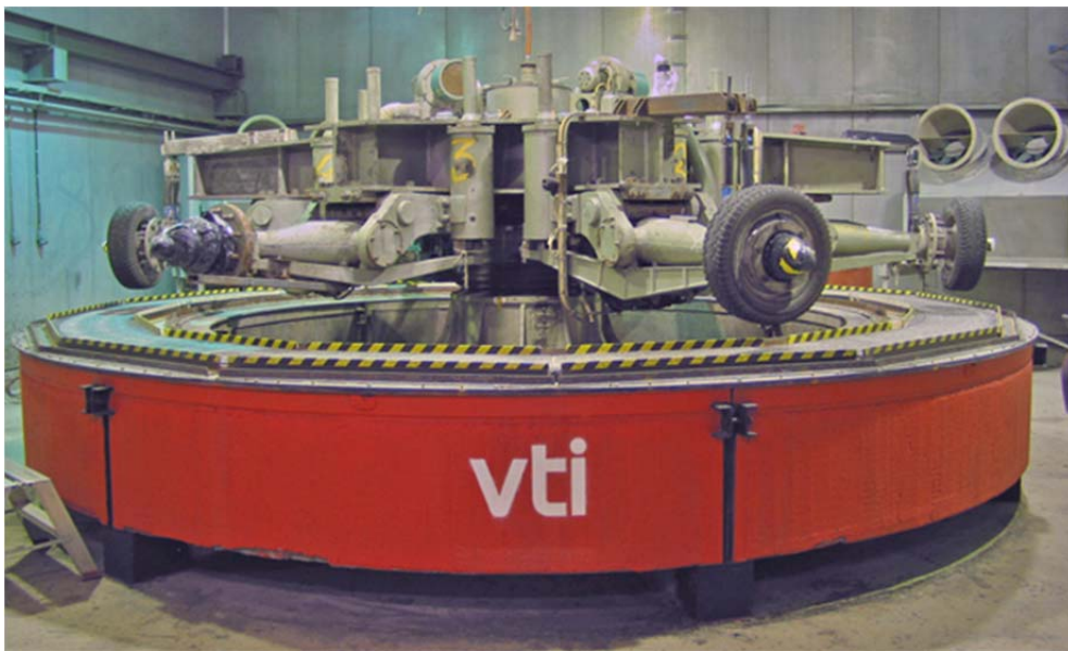
Figure 1 The VTI road simulator.
