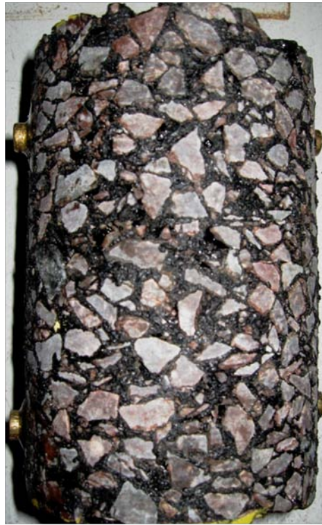
Figure B.2 – 19% Air void sample.
