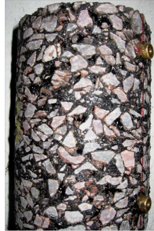
Figure B.3 – 21% Air void sample
