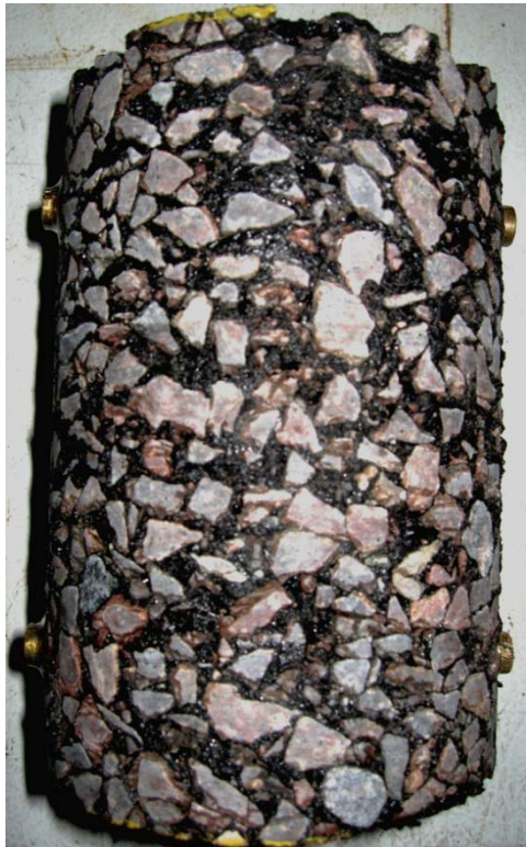
Figure B.1 – 17% Air void sample.
