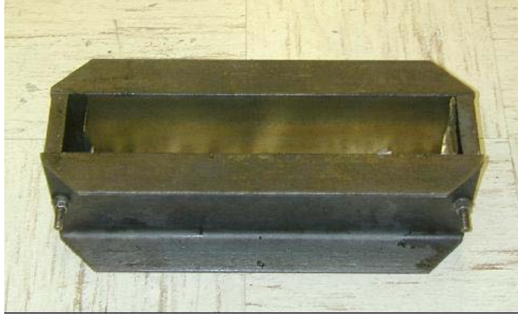
Figure 18 Manufactured Mold for Beam Compaction
