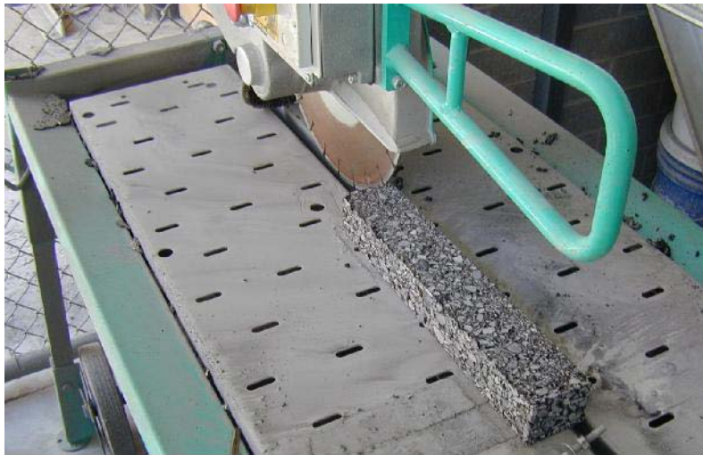
Figure 20 Beam specimen sawing.
