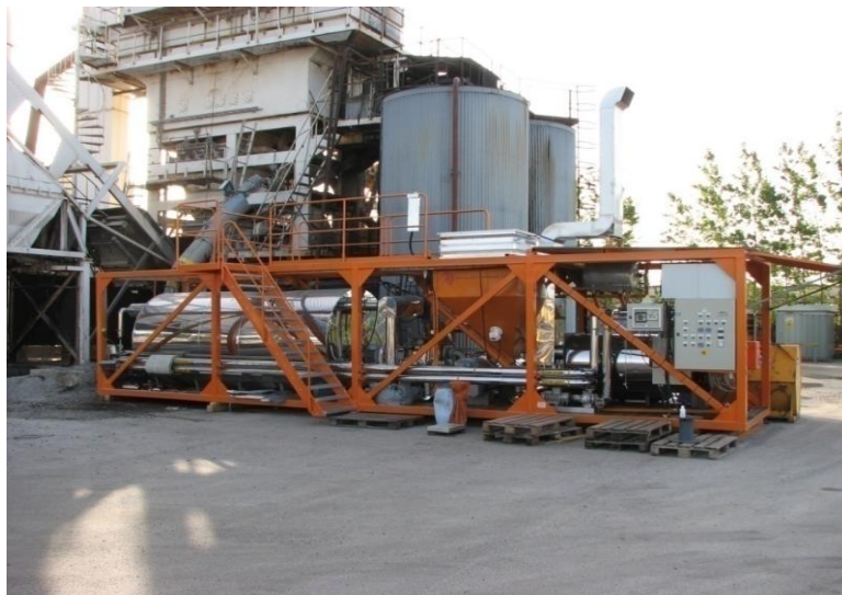
Figure 1. Mixing equipment connected to the asphalt plant
