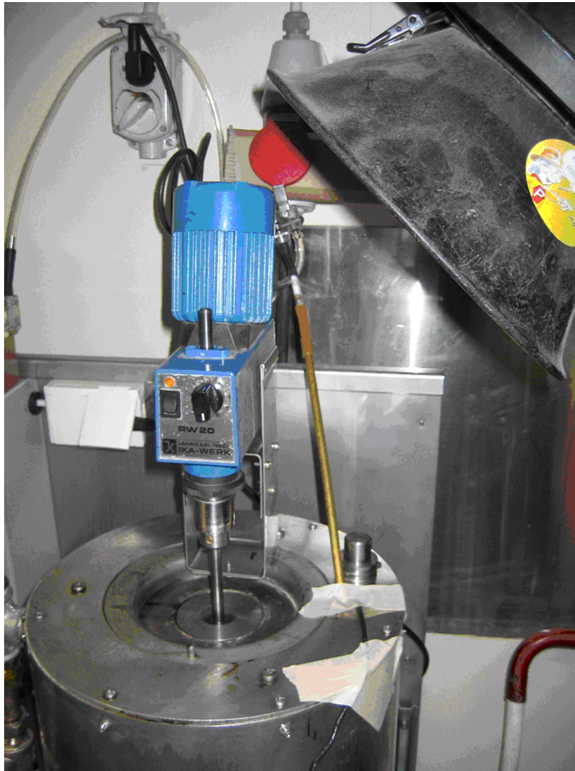
Pictures – Bitumen mixer used at the pilot study and Measurement 1 - 2007
